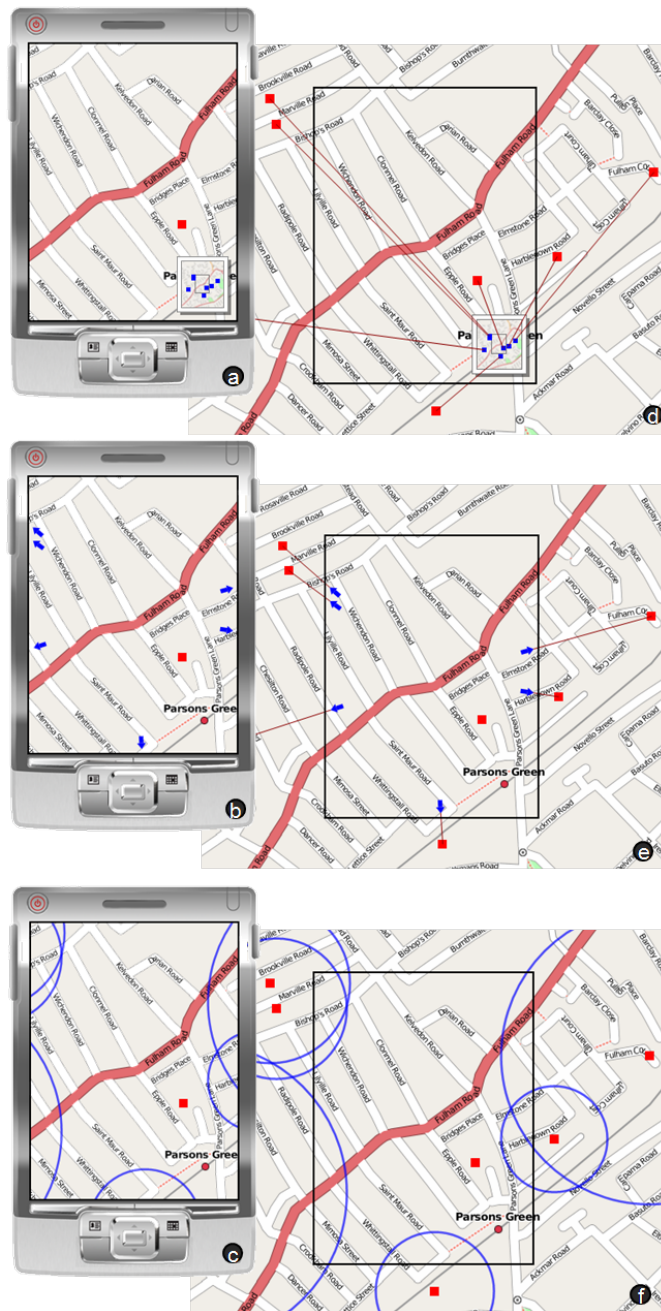
Figure 1: Three existing techniques for visualizing large datasets on a small device: a) overview+detail; b) arrows; c) Halo. Beneath (d-f) are larger sections of the map showing the off-screen locations with the respective visual techniques.
